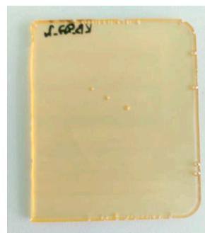
Fig. 6. 100% diBCB-DMS sample after primary heat treatment: 160°C — 5 h, 220°C — 1.5 h
