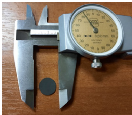
Fig. 5. Cold-sintered ceramic sample from (MnFeCoNiCu) 3 O 4 powder, relative density 0.71 (temperature 300°C, 0.1 wt % of NaOH).
