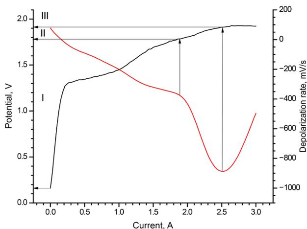
**Fig. 4.** Polarization and depolarization curves of GS32-VI alloy dissolution in the sulfuric acid electrolyte at a concentration of 100 g/dm<sup>3</sup>, 500 ms pulse duration, and a delay of 250 ms.
