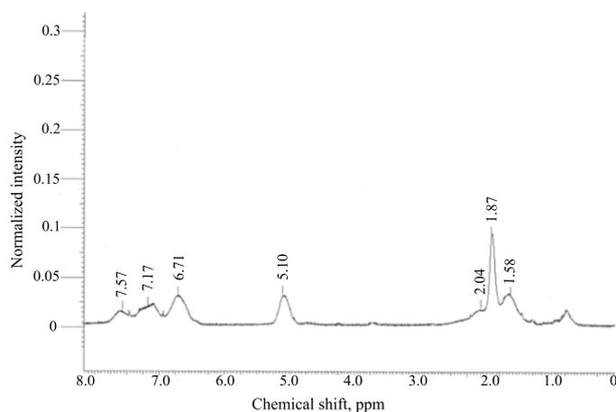
Fig. 1.  $^1\text{H}$  NMR spectrum of PVBAc in  $\text{C}_6\text{D}_6$ .
