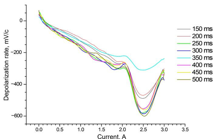
**Fig. 6.** Depolarization curves of GS32-VI alloy dissolution in a sulfuric acid electrolyte with a concentration of 100 g/dm<sup>3</sup>, a pulse duration of 500 ms, and different pause times.
