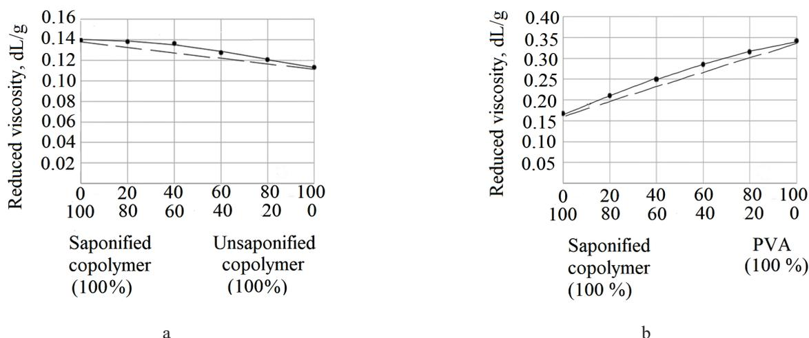
**Fig. 9.** Dependence of the reduced viscosity of the solutions on the composition of (a) saponified and unsaponified copolymer mixtures containing 16 mol % of styrene units, and (b) saponified copolymer mixtures containing 16 mol % of styrene units with PVA. The solvent is 1,4-dioxane,  $30^{\circ}\text{C}$ . The concentration of the polymer mixture, g/dL: (a) 1 and (b) 2.
