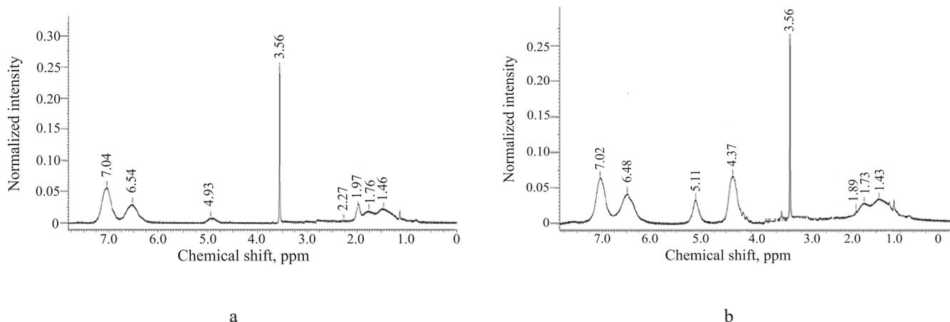
**Fig. 3.** <sup>1</sup>H NMR spectra of dissolved in DMSO-*d*<sub>6</sub> (a) styrene copolymers (82 mol %) containing VBAC (2 mol %) and VBA (16 mol %) units and (b) VBAC copolymers (3 mol %) containing VBA (97 mol %) units.
