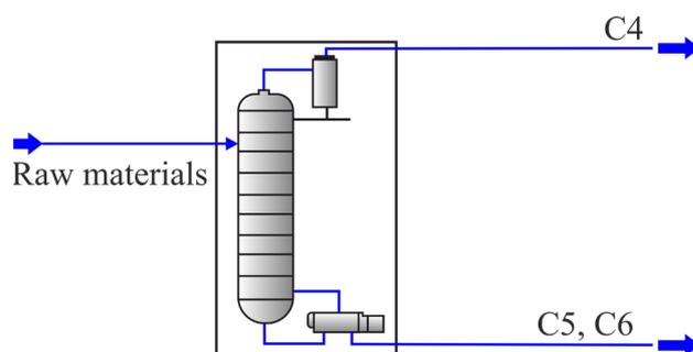
Fig. 2. Diagram of the debutanizing column.
