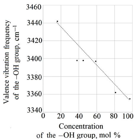
**Fig. 5.** Dependence of the maximum of the 3442–3355 cm<sup>-1</sup> band in the IR spectra of saponified VBAC copolymers with styrene on the content of VBA units in them.
