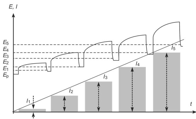
**Fig. 1.** Current diagram for polarization and depolarization curves.
