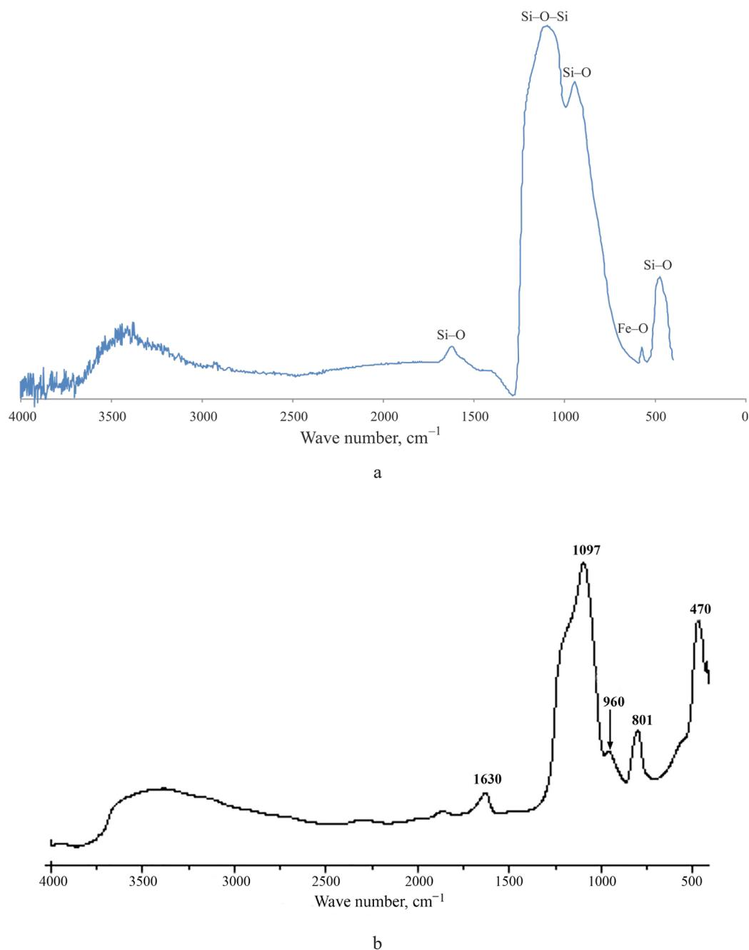
**Fig. 1.** FTIR spectrum of (a) the studied nc-Si/SiO<sub>2</sub>/Fe sample (0.3 mass % in KBr) and (b) the aerosil sample (powdered SiO<sub>2</sub> with a particle size of 15 nm).
