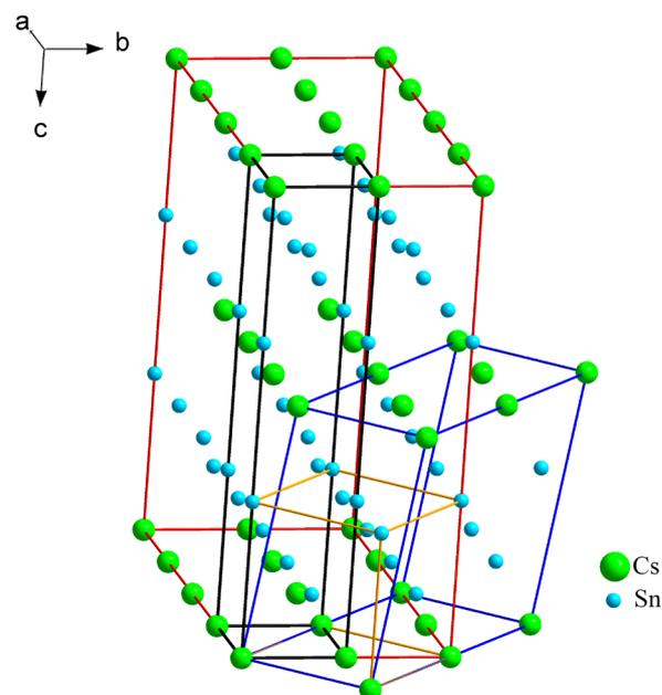
**Fig. 4.** Transformation of the unit cell of  $\text{CsSn}_2\text{F}_5$ : fluorine atoms are removed from the model; black tetragonal cell according to [11] (the coordinate system is for this lattice); red orthorhombic cell according to [10]; the orange cubic cell is fluorite-like cell; the blue monoclinic cell is obtained by the indexing results.
