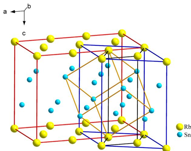
**Fig. 3.** Transformation of the unit cell of  $\text{RbSn}_2\text{F}_5$ : fluorine atoms are removed from the model; black hexagonal cell accords to [11] (the coordinate system is for this lattice); red orthorhombic cell accords to [10]; the orange cubic cell is fluorite-like cell; the blue hexagonal cell is obtained by the indexing results.
