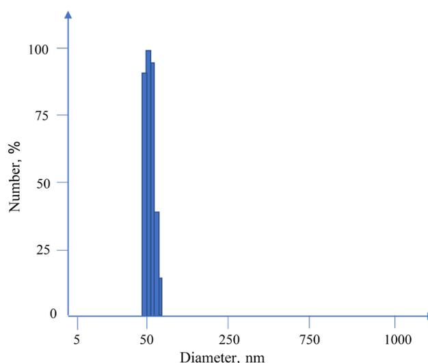
**Fig. 2.** Molecular weight distribution of modified nc-Si/SiO<sub>x</sub>/Fe-citric nanoparticles (1%). The average hydrodynamic diameter was 57 nm.
