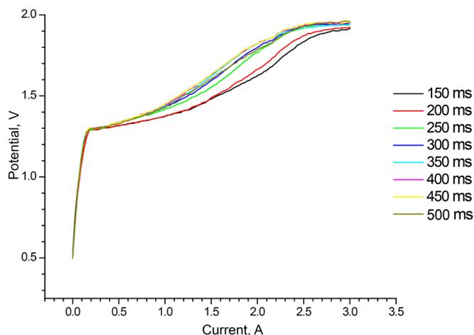
**Fig. 5.** Polarization curves of GS32-VI alloy dissolution in a sulfuric acid electrolyte with a concentration of 100 g/dm<sup>3</sup>, a pulse duration of 500 ms, and different pause times.
