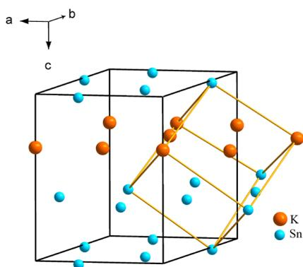
**Fig. 2.** Transformation of the unit cell of  $\text{KSn}_2\text{F}_5$ : fluorine atoms are removed from the model; hexagonal cell accords to [7] (the coordinate system is for this lattice); orange cubic cell is fluorite-like cell.
