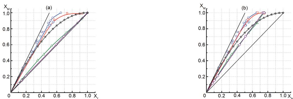
**Fig. 3.** Dependences of monomer conversion ( $X_m$ ) on functional groups conversion ( $X_f$ ) (a) and of monomer conversion ( $X_m$ ) on the “reduced” conversion of functional groups ( $X_{fm}$ ) (b) for (★) statistical assembly according to Flory, (○) –  $(\text{CH}_3)_2\text{Si}(\text{OH})_2$  HMFC, partial hydrolysis (□) –  $(\text{CH}_3)_2\text{Si}(\text{OCH}_3)_2$ , (△) –  $(\text{CH}_3)_2\text{SiCl}_2$  and (◇) –  $(\text{CH}_3)_2\text{Si}(\text{OCOCH}_3)_2$ .
