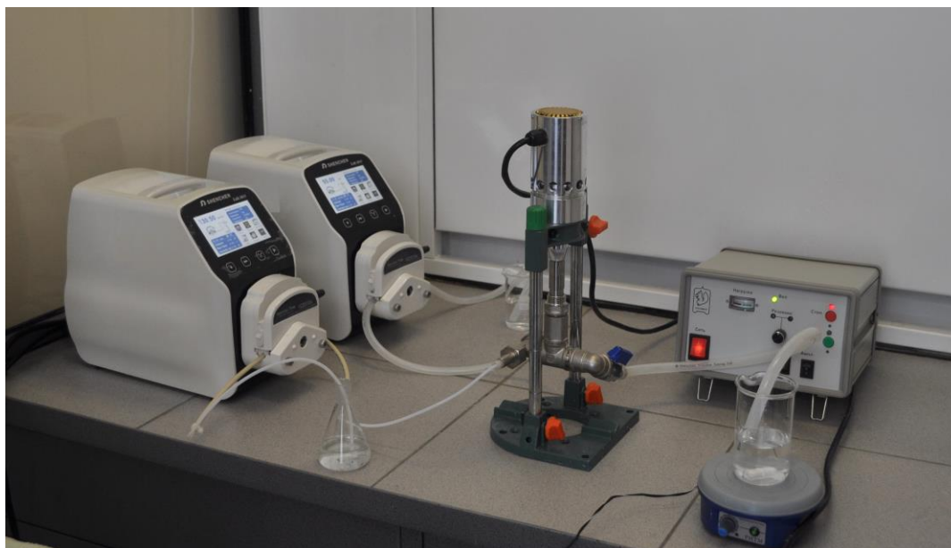
Figure 2. Installations for obtaining polymeric particles based on MOD MEF 92 ultrasonic flowing homogenizer.
