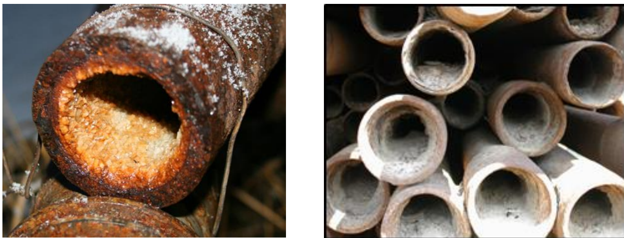
Figure 6. Pumping and compression pipes for oil production polluted by internal deposits of \text{Ba}(\text{Sr}, \text{Ra})\text{SO}_4 with natural radionuclides coprecipitated from stratum water.
