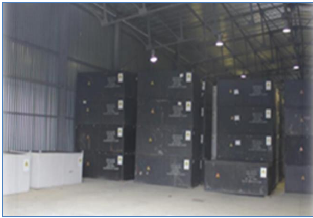
Figure 3. Temporary storage of containerized SRW in easily built constructions.
