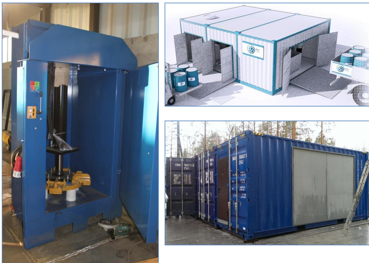
Figure 2. Mobile complex of FSUE “RosRAO” for sorting, fragmenting and prepressing SRW in 200 dm 3 barrels.
