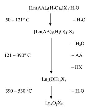
The thermogravimetric data confirm the existence of outer-sphere water weakly bonded in the crystalline structure of the complex compounds.
