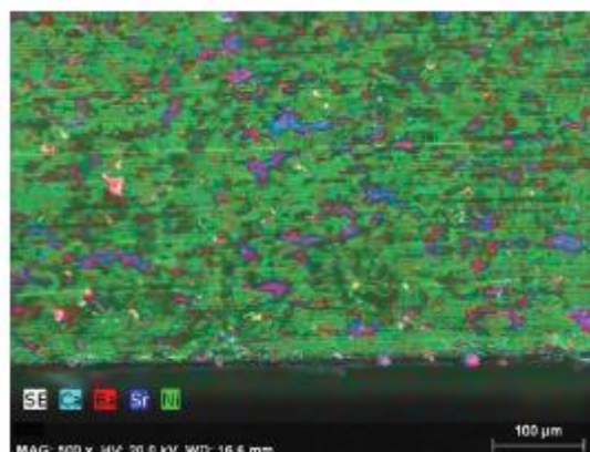
Figure 6. Mapping of the cylindrical surface of an oxide-nickel emitter produced with the use of agglomerates.
