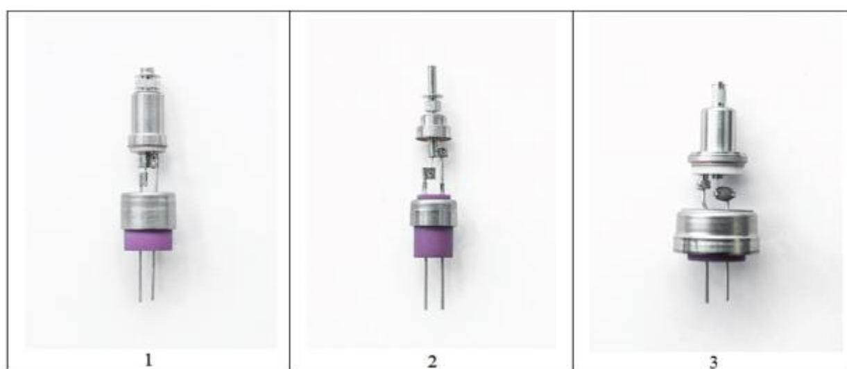
Figure 10. Cathode-preheating blocks with emitters based on oxide-nickel cathode materials: 1 – M1 type product; 2 – M2 type product; 3 – M3 type product.
