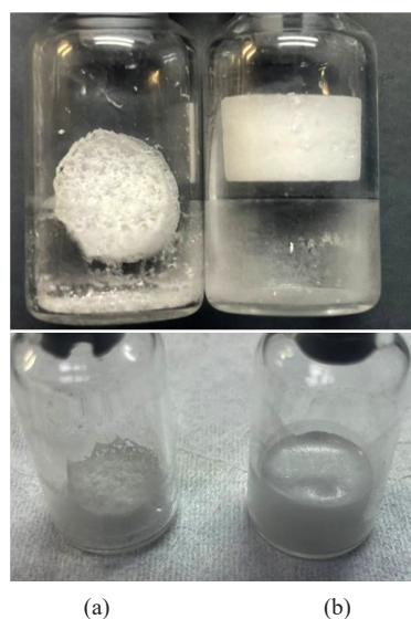
Fig. 1. An appearance of the cakes after drying of the samples. (a) 4% trehalose with NaCl; (b) 4% trehalose without NaCl
