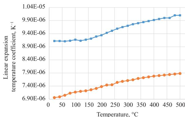
**Fig. 6.** Dependence of the matrices thermal expansion coefficient on temperature (squares, blue line—a matrix with a pyrochlore structure; circles, a red line—a matrix with an orthorhombic REE titanate structure)
