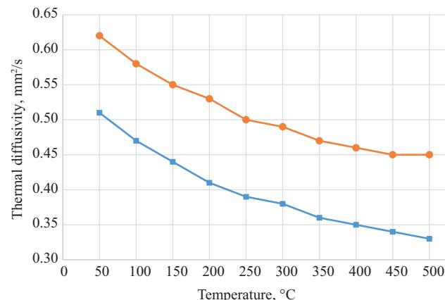
**Fig. 4.** Dependencies of the crystalline matrices thermal diffusivity on temperature (squares, blue line—a matrix with a pyrochlore structure; circles, red line—a matrix with structure of an orthorhombic REE titanate)
