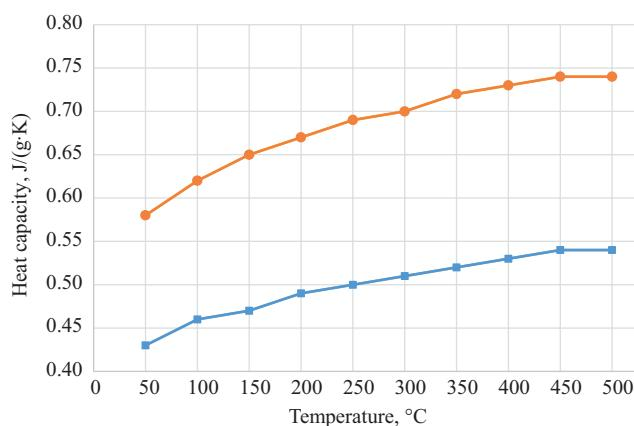
**Fig. 3.** Dependencies of the crystalline matrices heat capacity on temperature (squares, blue line—a matrix with a pyrochlore structure; circles, red line—a matrix with structure of an orthorhombic REE titanate)
