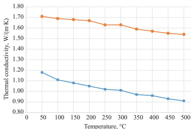
**Fig. 5.** Dependencies of the thermal conductivity coefficients of crystalline matrices on temperature (squares, blue line—a matrix with a pyrochlore structure; circles, red line—a matrix with structure of anorthorhombic REE titanate)
