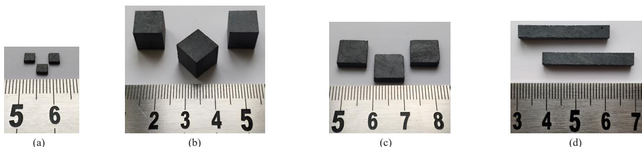
**Fig. 1.** Appearance of MLMs samples of various sizes: (a) heat capacity determining samples; (b) compressive strength determining samples; (c) thermal diffusivity determining samples; (d) ultimate strength in bending determining samples
