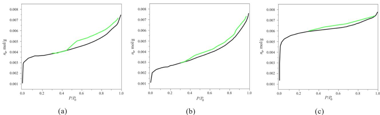
**Fig. 5.** Adsorption–desorption isotherms of N<sub>2</sub> by nanoparticles isolated from cobalt complexes of glucose (a), glycogen (b), and sucrose (c).  $n_a$  is the amount of adsorbed substance, mol·g<sup>-1</sup>;  $P/P_0$  is the relative pressure (ratio of system pressure to condensation pressure).
