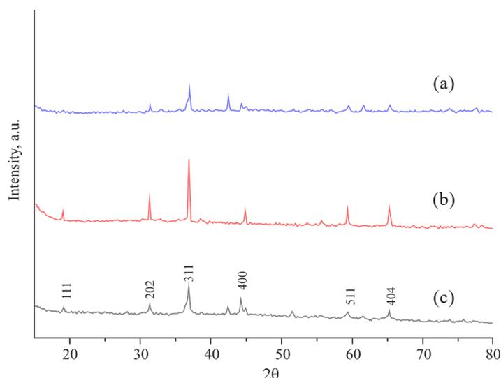
Fig. 2. X-ray diffraction patterns of oxide phases obtained by calcination of cobalt(II) complexes with sucrose (a), glycogen (b), and glucose (c).
