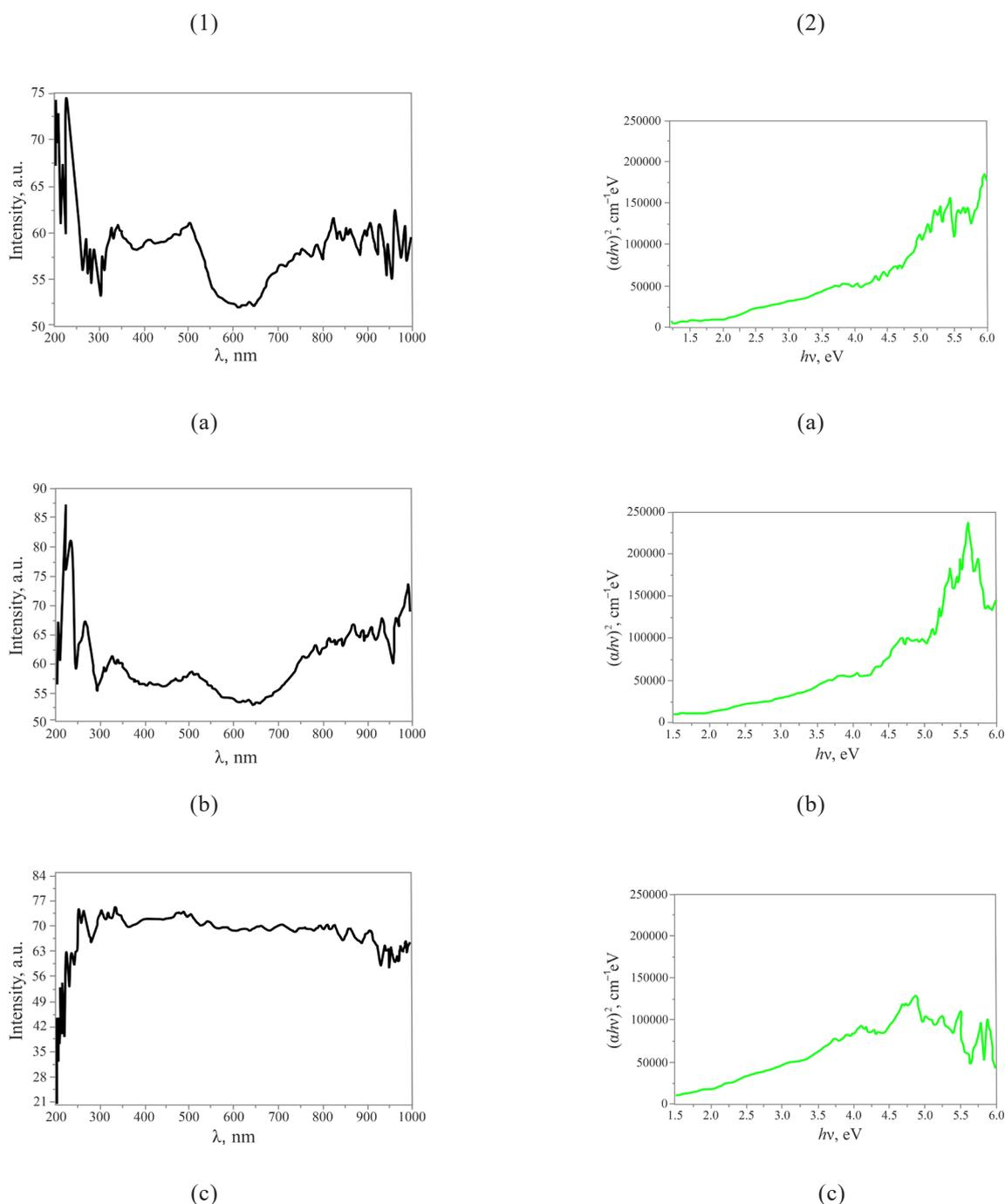
**Fig. 7.** Electronic absorption spectra (1) and band gap (2) of  $\text{Co}_3\text{O}_4$  nanoparticles isolated from cobalt complexes of glucose (a), glycogen (b), and sucrose (c);  $(\alpha h\nu)^2$  is the absorption coefficient squared,  $\text{cm}^{-1}\cdot\text{eV}$ ;  $h\nu$  is the photon energy, eV.
