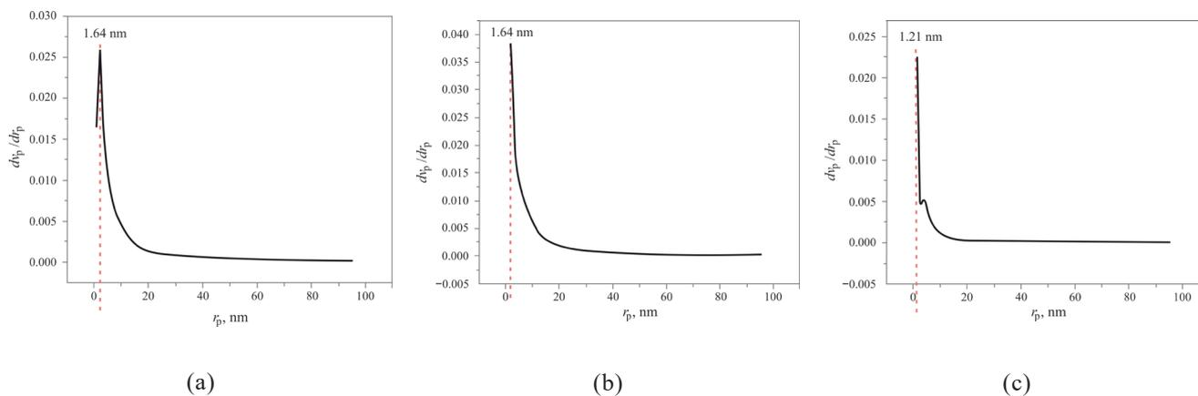
**Fig. 6.** BJH analysis of  $Co_3O_4$  nanoparticles isolated from cobalt complexes of glucose (a), glycogen (b), and sucrose (c);  $dV_m/dr_p$  is the derivative of the ratio of specific volume to average pore radius,  $r_p$  is the pore radius, nm.
