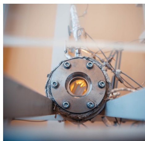
Fig. 3. (a) Sketch of the high pressure apparatus: (1) inspection windows; (2) pressure flange; (3) inlet connections; (4) outlet connections. (b) External view of the apparatus from the side of the inspection window.
