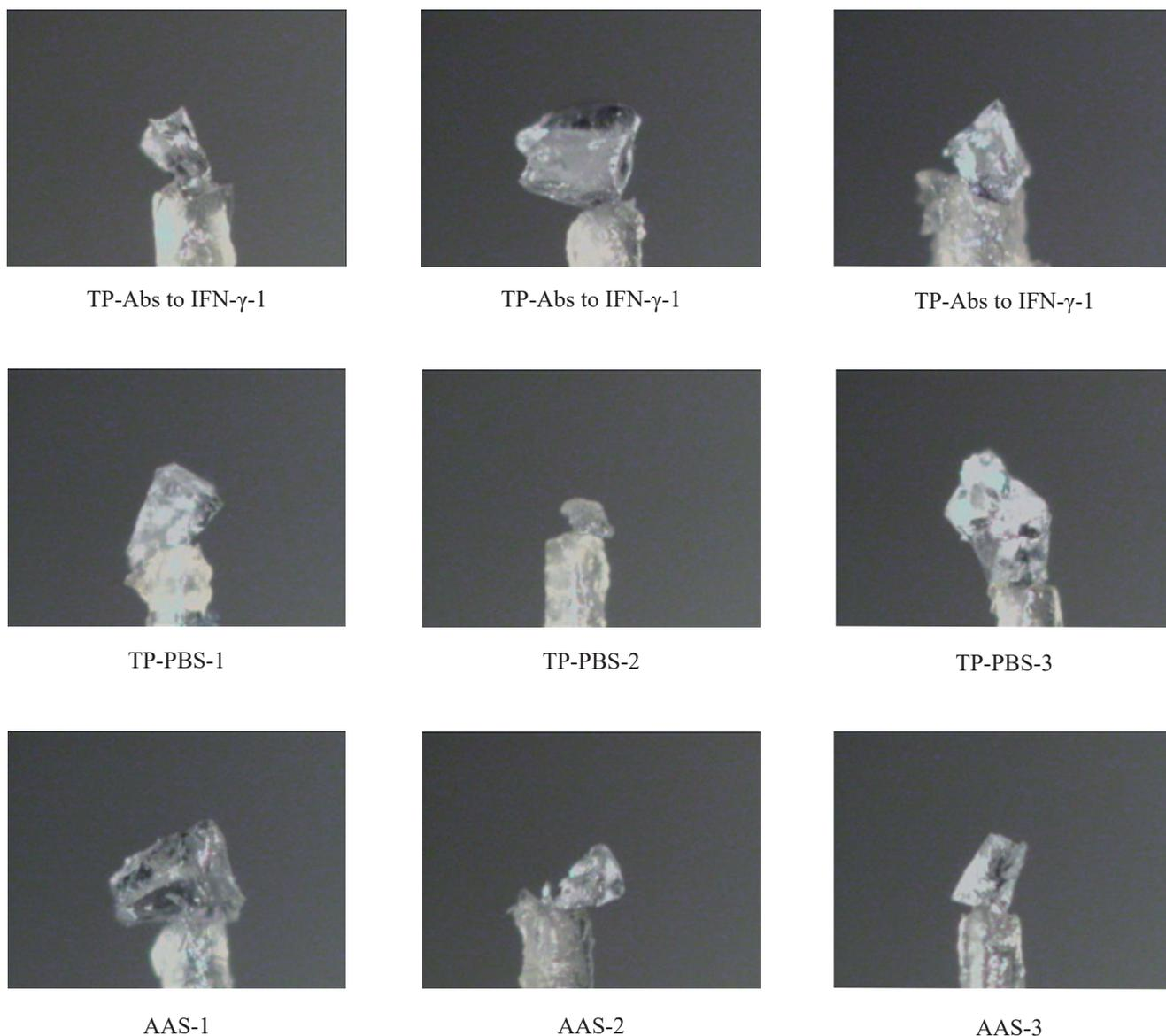
**Fig. 2.** Photos of TGS crystals pasted on a glass thread for conducting XRD.
