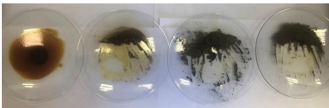
Fig. 5. Oil sludge sorption on a hard surface: from left to right: oil product sample, quartz sand, calcined sorbent, and modified sorbent.
