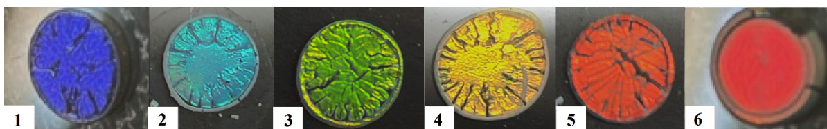
Fig. 1. Photographs of photonic colloidal crystals (PCCs) from polystyrene microspheres of different diameters: (1) 180 nm, (2) 200 nm, (3) 220 nm, (4) 230 nm, (5) 240 nm, (6) 260 nm.
