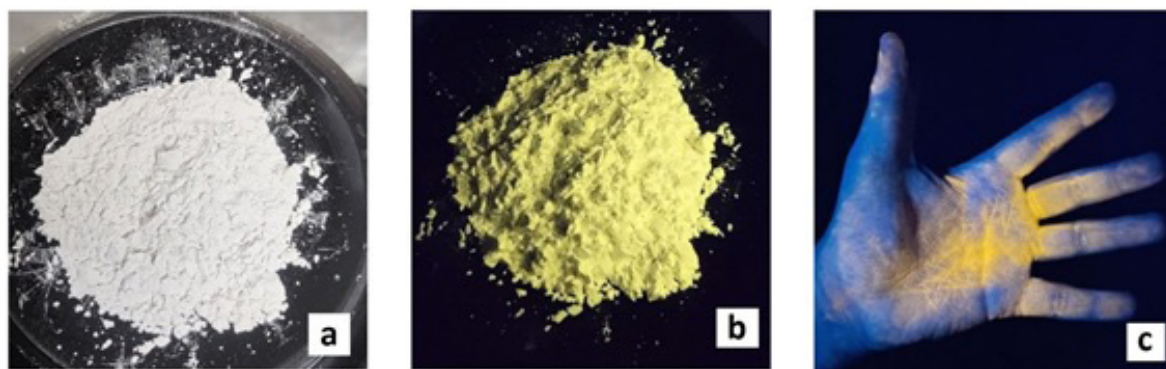
Fig. 5. Samples of reduced phosphogypsum under illumination: ordinary light (a), ultraviolet light (b, c), and ultraviolet light with a light filter (b).
