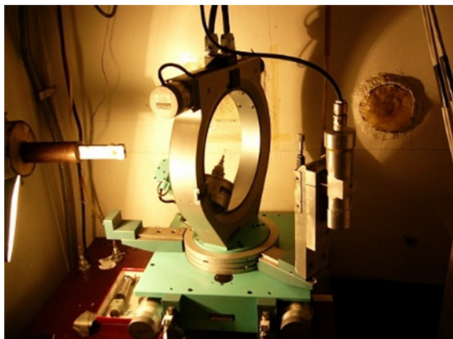
Fig. 2. HUBER 511/424 goniometer with vertical “side” detector in the “house.”
