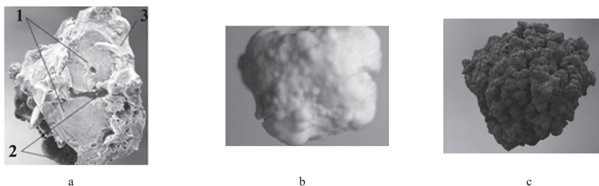
**Fig. 5.** Fraction 1.00–1.99 mm: (a) granule from Experiment 10; (b) granule from Experiment 11; (c) granule from Experiment 12. At Fig. a: 1 – contaminated soil, 2 – pitch, 3 – deposits of salts containing heavy metals.
