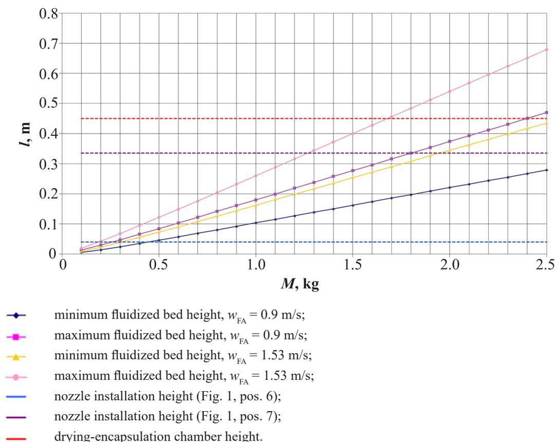
Fig. 2. Calculated dependence of the fluidized bed height on its mass ( $d_p = 0.5$  mm).
