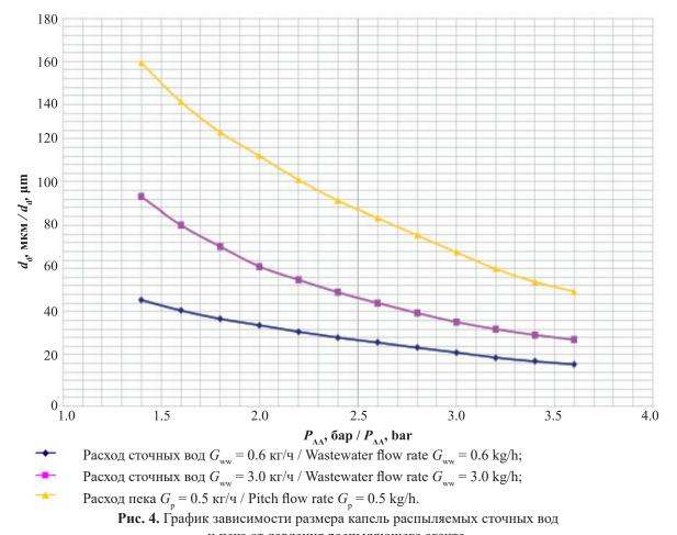
и пека от давления распыляющего агента. **Fig. 4.** Calculated dependence of the droplet size of sprayed wastewater and pitch on the pressure of the atomizing agent.
