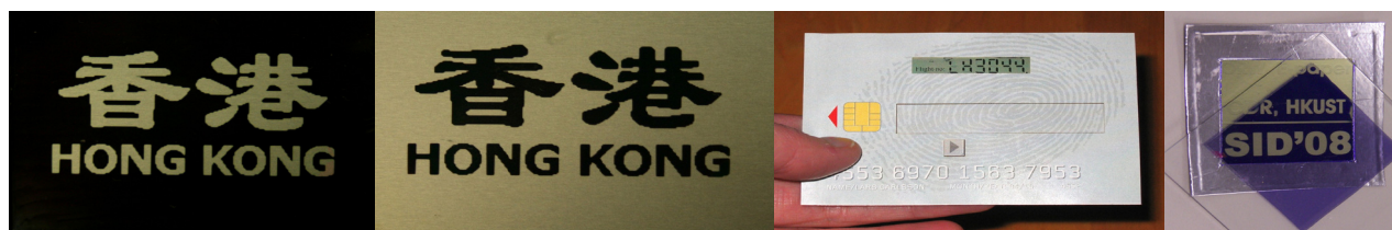
Fig. 3. Left to right: ORW E-paper for advertisements, plastic cards and security applications.
